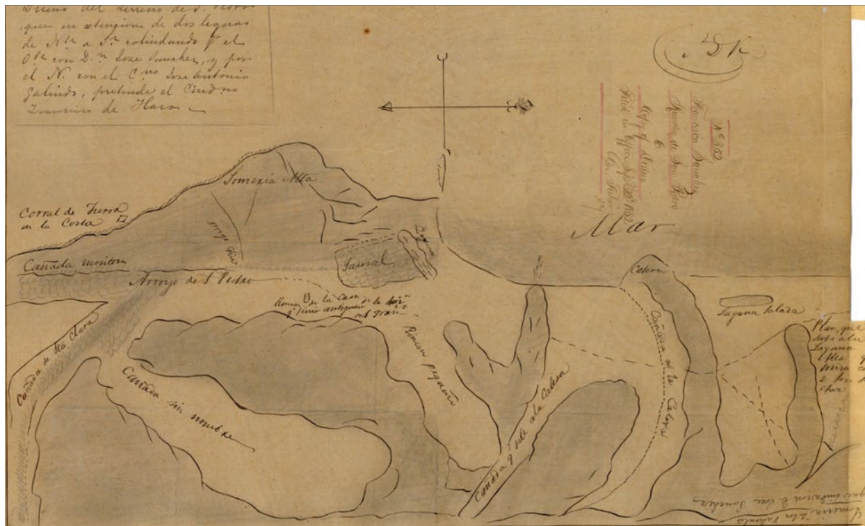
Figure 4 Diseño of San Pedro, undated, showing the landscape and trails through the Mexican 1839 land grant. To obtain a land grant during the Mexican period, the applicant accompanied the petition with a topographical sketch or diseño. Mexican law did not require precision surveying. The technique involved in making a diseño was that of the ability to stay in the saddle, to read a magnetic compass, and to measure the distance between two points by means of a rawhide cord tied between two poles; the processing was carried out with pencil, quill pen, ink and water color. San Pedro is located to the left of center, showing a valley with trail and swampy lagoon.
